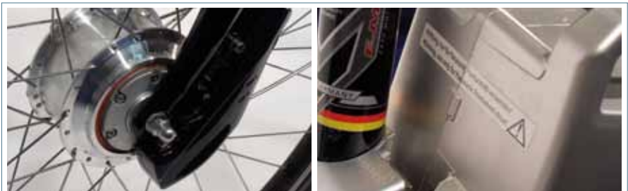
The front wheel hub motor of Panasonic is almost just as big as a hub dynamo. • The battery of the Agattu F may not be exchanged with the battery of an Agattu C with bottom bracket motor.
