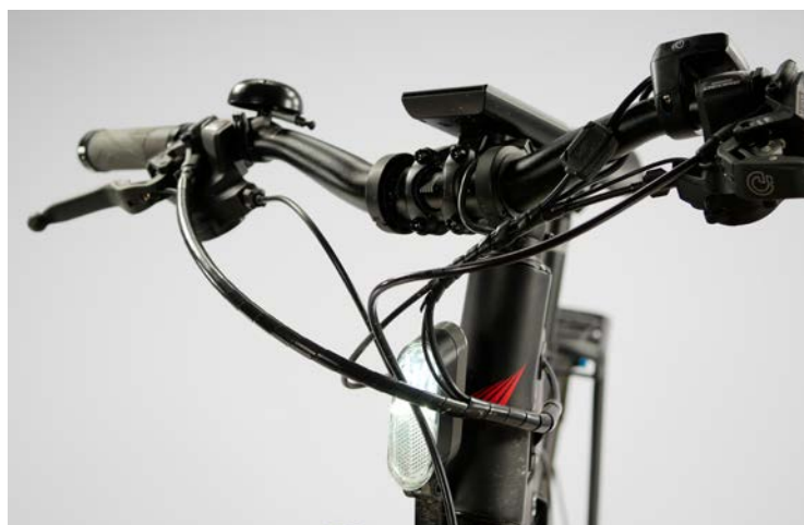
LEFT The Trelock front light shines brightly, but unfortunately there are always wires, hoses and Bowden cables between it and the road, no matter how you twist and turn the handlebars. Not a problem exclusive to Haibike, but it’s particularly noticeable here, because the front light is fitted so close to the headtube.
