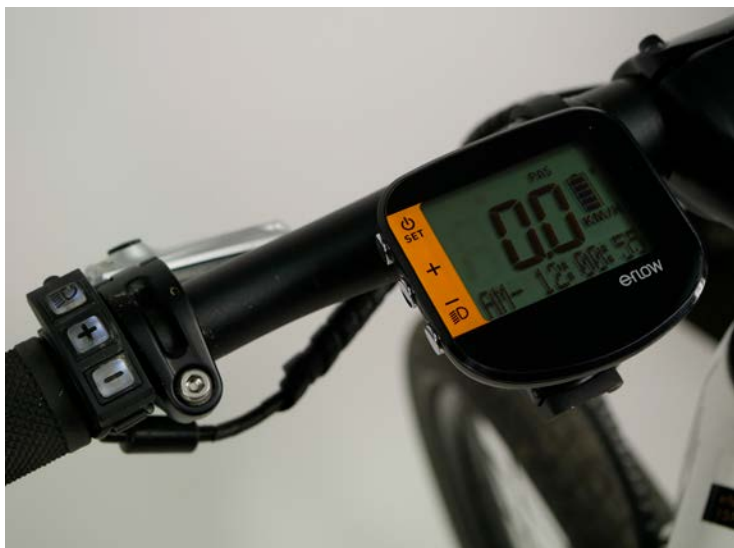
LEFT The removable control unit for the eflow ER2 limits itself to the usual functions of a cycle computer, for example total km, ride km, average km/h, max km/h, and battery capacity and power assist level are also shown. This display is operated with your thumb via a backlit button unit, so you do not have to remove a hand from the handlebars.
