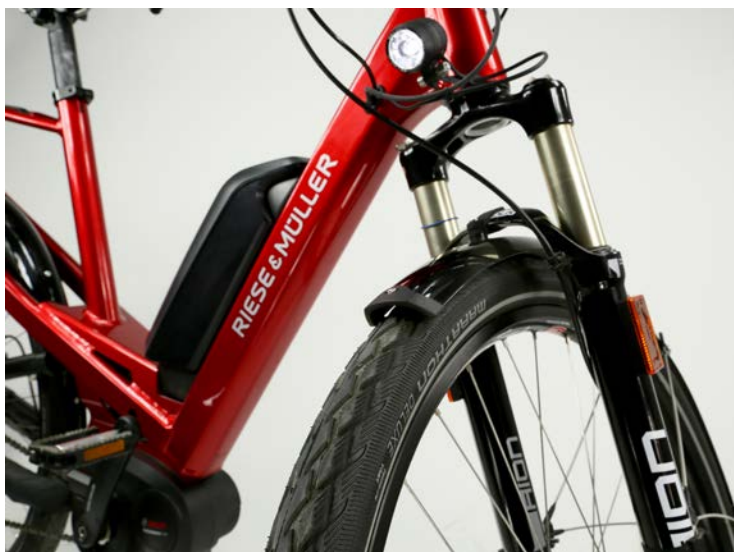
LEFT Full fat: the Schwalbe Marathon Deluxe tyres are a hybrid of the well-proven Marathon model and the comfortable shock-absorbing Big Apple tyre. The Suntour Aion suspension fork has plenty of travel too, and it is equipped with a through-axle system and the orange side reflectors which are mandatory in Germany for pedelecs 45.
