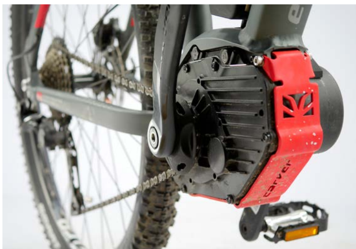
LEFT The Bosch mid motor in a rare minimalist installation - without any of the rather absurd-looking Tupperware effect of the usual plastic fairings. Carver has sensibly left these off, and just installed a red metal plate as a bashguard around the motor assembly, giving protection against hard landings off-road.
