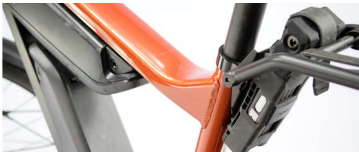
LEFT Practical: the Bordo folding lock from ABUS, which fits neatly behind the seatpost when you're riding. Even more practical: the key for the ABUS fits both of the batteries as well as the bike lock.
