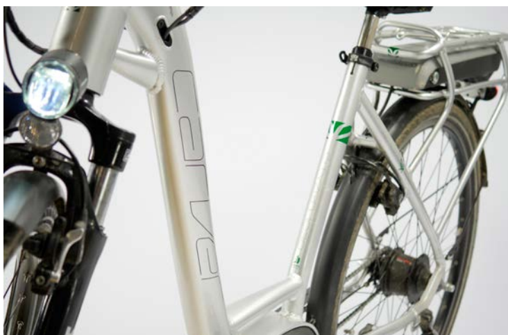
LEFT Depending on the stature of the rider, some undesirable flex of the frame can occur, despite the massive frame tubing. The cross-beam above the mid motor only works as a carrying handle for people with thin fingers, and even then it's not pleasant to use with thick winter gloves.
