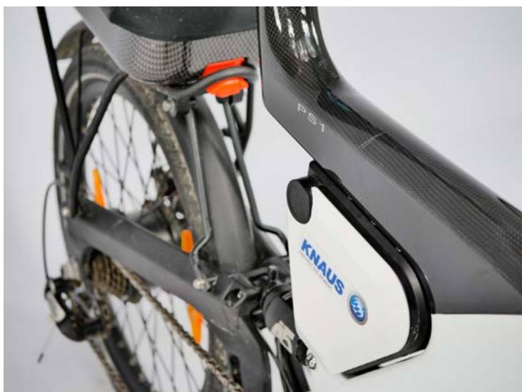
LEFT The carbon fibre frame completely encloses the battery. With a capacity of just 238 Wh this is one of the smallest on test, in terms of its weight as well as its capacity. But despite the use of carbon fibre, this pedelec from Knaus still weighs 20.2 kg.
