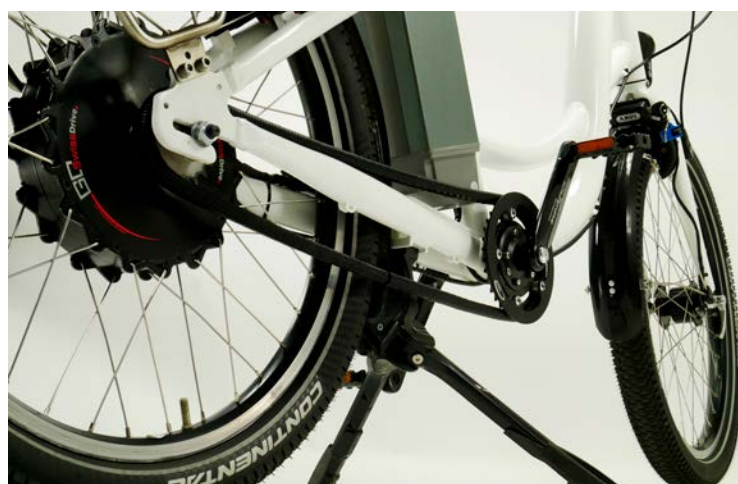
LEFT A powerful motor and the two speeds from the bottom bracket gearbox are perfectly adequate and, together with the chain protected by its plastic sleeve, promise years of low-maintenance service. Operating the two speed gearshift with your heels takes a little getting used to, but after some practice it feels perfectly natural.
