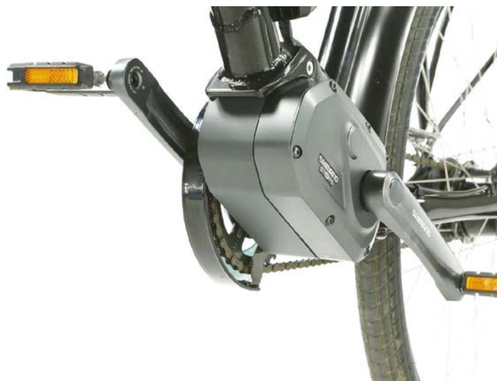
LEFT The Shimano Steps mid motor system is, rather like several other mid motor systems, attached to the frame with three bolts as a sort of 'foreign body'. When shifting gear using the automatic gear change, the drive power from the motor is automatically dropped for the brief instant of shifting, so that on hills, the gear changing process works quickly and without much gear wear.
