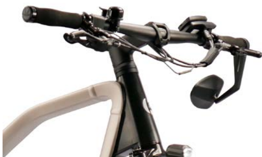
LEFT An exemplary tidy handlebar! All cables disappear into the stem, and so are protected against damage. Furthermore, unlike the case on numerous other bikes, they do not flop around into the beam of the front light.
