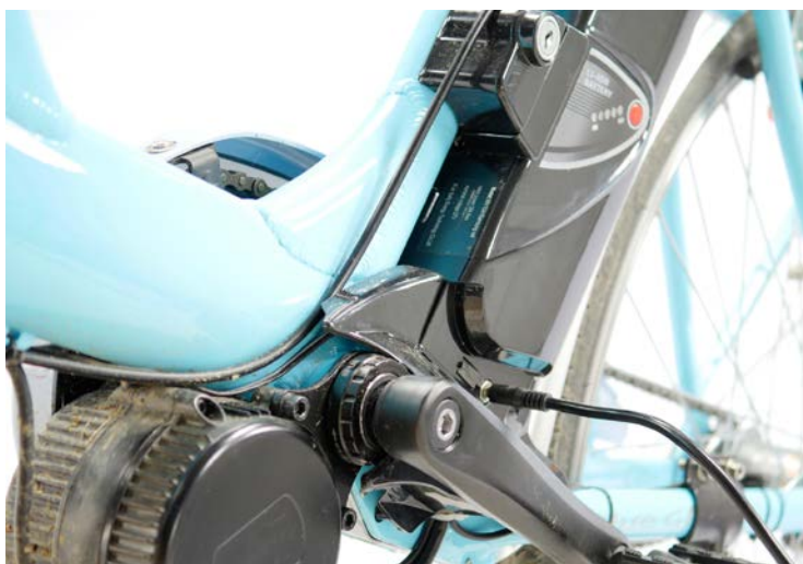
LEFT The Bafang mid motor, which assists with the pedalling almost silently, hangs somewhat underwhelmingly under the standard bottom bracket. The battery behind the seatpost, which looks rather like a plump and poorly made copy of the Panasonic battery packs, also irritated the test riders with its continuous rattling.
