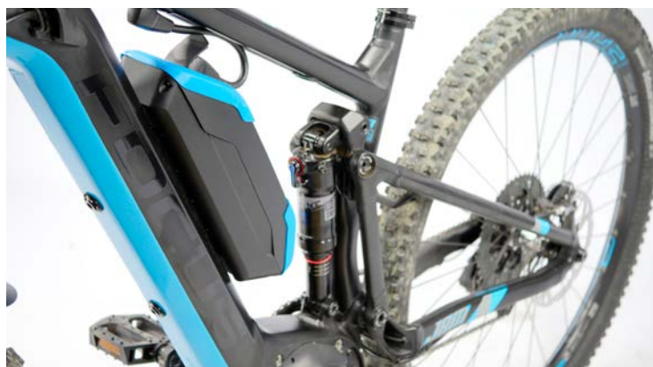
LEFT The optional extra battery doubles the climbing range from 917,5 to 1835 vertical metres. The securely fixed battery in the lower frame tube can only be charged by direct connection to the charger, while the extra battery is easily removable. When the extra battery's cable is plugged it, it is always discharged first.
