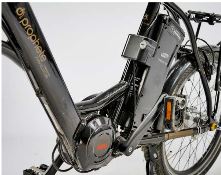
LEFT Showing off the big brandnames: Samsung battery pack and AEG motor. These components are not however integrated all that harmoniously, and the cables are also arranged rather wildly. Like Henry Ford's Model T from 1924, it comes in any colour you like, so long as it's black.
