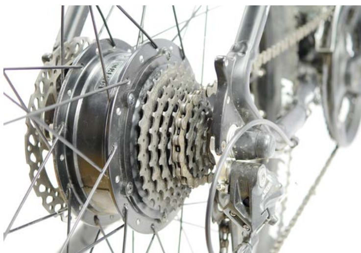
LEFT The hub motor from Bafang is powerful and, despite being geared, quiet. It provided strong assistance on all of the test sections: city, hills and tour. It is just unfortunate that to save money they have omitted a torque sensor, which means that sometimes the motor kicks in rather suddenly and boisterously.
