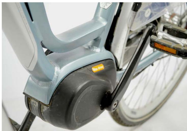
LEFT The Bafang MAX Drive mid motor distinguishes itself by being very powerful yet still very quiet. This was something that many test riders really appreciated, especially while riding through the countryside on the Tour route.
