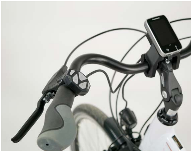
LEFT Height-adjustable stem, swept-back handlebars and ergonomic grips were all appreciated by the testers. The Magura hydraulic rim brakes provided good stopping, with silky-smooth modulation. The central display for the power assist system has a USB port to supply power to other electrical devices, for example a mobile phone or a GPS navigation system.
