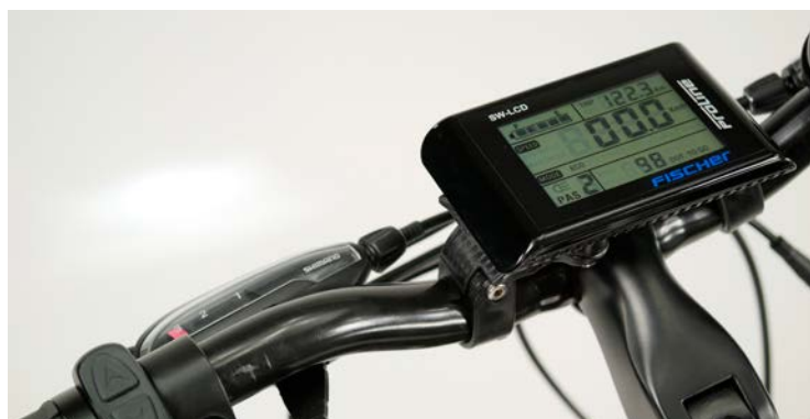
LEFT The cockpit of the Fischer Proline Trekking ETD 1606, with a multi-functional display mounted fixed to the bike. The USB charge function on the display is self-explanatory and is a must-have for digital nomads. The functions, including the lights, can be easily operated with the thumbs, without taking a hand from the bars. You get masses of functions here for very reasonable money.
