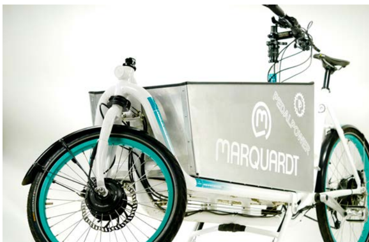
LEFT With its double cable operated steering, the front wheel can turn to extreme angles of lock either side. This is less relevant while riding than it is when parking, where it allows you to manoeuvre efficiently even in very tight spaces. The all wheel drive system from Marquardt impressed with its huge reserves of power.
