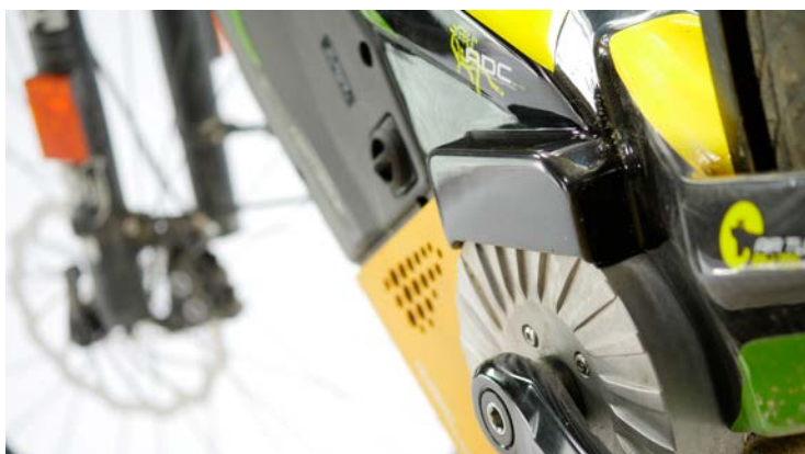
LEFT Characteristic of M1 is the powerful TQ mid motor, which propelled the Sterzing Commuter MCF to a uniquely high U-factor among the bikes on test: 3.88 for the touring circuit. The rather bulky and awkward to change battery needs recharging after about 50 km on the "Tour" route.
