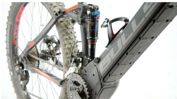
LEFT Once you've worked out how to remove the battery in a downwards direction it's very easy. However, after a test ride the battery was by some way the most dirty part of this offroad pedelec: it is sprayed beautifully by the muck from the front wheel... so before charging the battery it's probably worth giving it a good clean.
