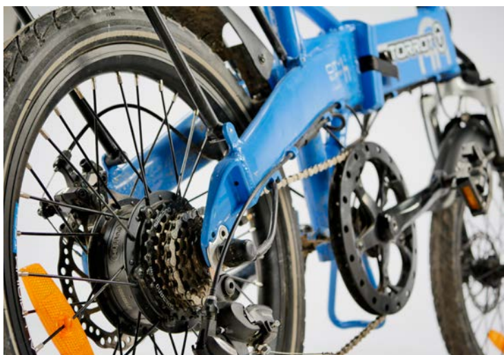
LEFT The engine room: this compact but very potent hub motor from Bafang produces power assist factors higher than you would expect from a folding bike. It's hard to understand why old-fashioned orange reflectors are fitted to the wheels when the tyres have reflective strips.
