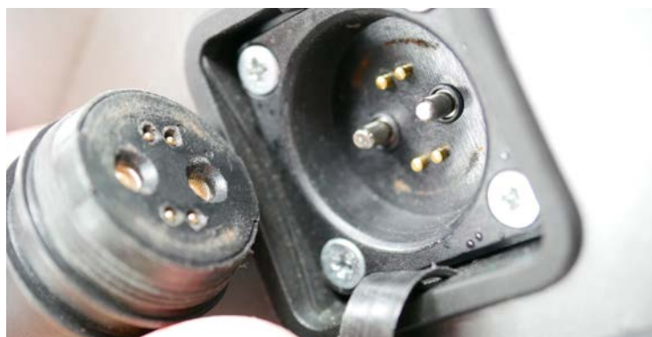
LEFT What makes the Stromer ST2 S special is the well-considered application of industry-standard interfaces: pictured here is the universal charging port complying with the future standards IEC 61851-3-2 / DIN IEC/TS 61851-3-2 (VDE V 0122-3-2). But also on the Stromer ST2 S are GSM for mobile internet connection, GPS for position location and Bluetooth for connection with additional mobile devices.
