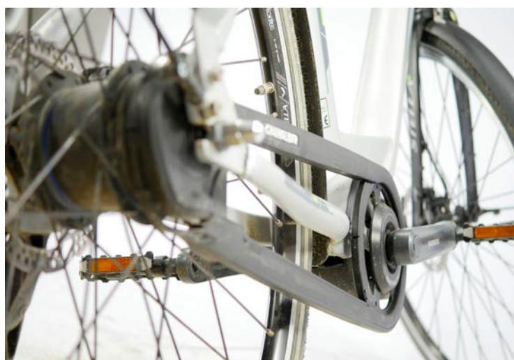
LEFT The Shimano Steps motor is restrained in its design, and here it is excellently combined with the "Chainglider" chain guard. This not only keeps your trousers free of chain lubricant; it also promotes a longer service life for the chain and sprockets.
