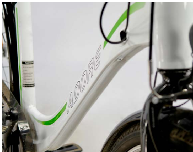
LEFT The frame was presumably meant to look rather elegant and sophisticated, because it's made from elaborately manufactured, complex-shaped tubing. But a completely normal round tube would quite likely have delivered improved stability. The shape of the tube they have used provides little lateral rigidity, rather like a plank standing vertically on one edge.
