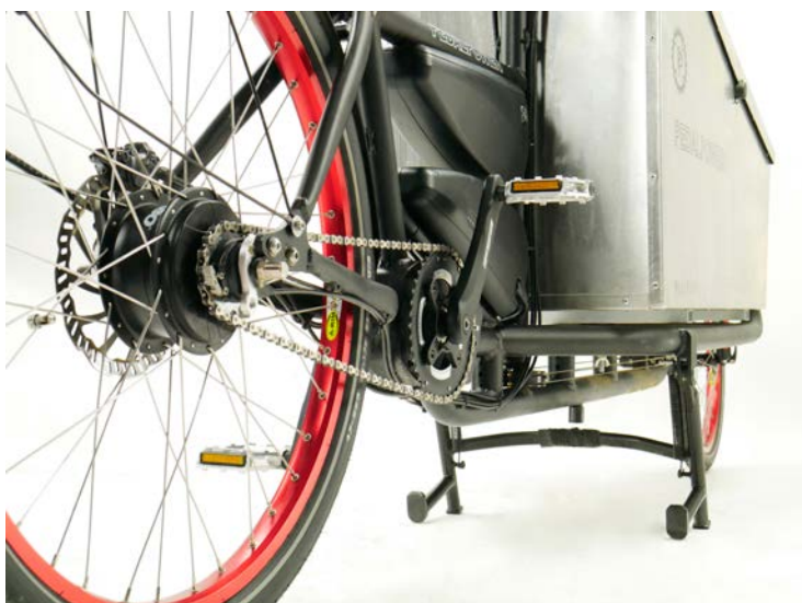
LEFT Masses of technology in not much space: two batteries almost completely fill the frame of the “Pedalpower eHarry”. The “Brose” motor assists your pedalling quietly but powerfully – and the motor power, together with your muscle power, is transferred to the rear wheel by the NuVinci step-less hub gear.
