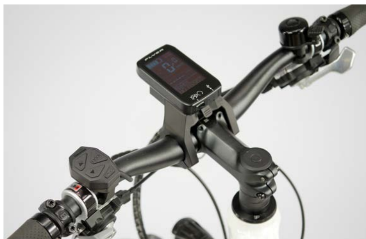
LEFT The cockpit is typical Flyer: super solid and functional. On the left, the shifter for the 3-speed hub gear, and on the right, for the 9-speed derailleur. The Panasonic display, and the controls, are intuitive to operate. The push assist is very powerful, assuming you've shifted to lowest gear in advance.
