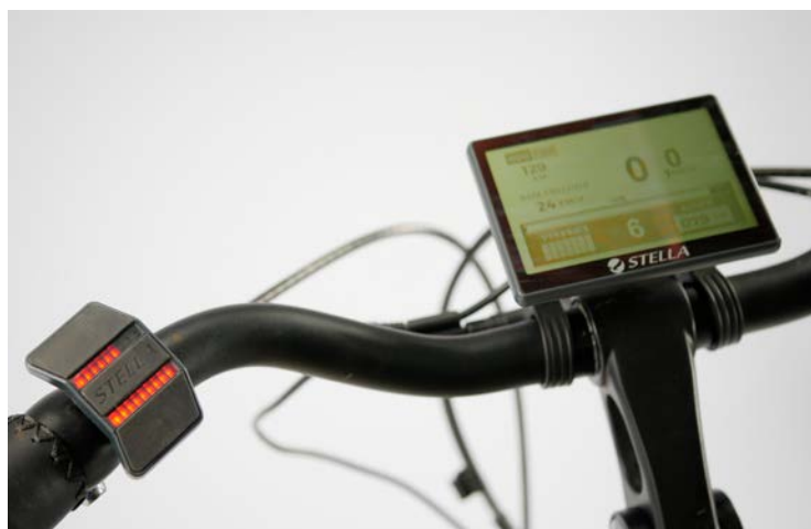
LEFT One of the best details: the remote control station with red Knight Rider moving lights – it’s just a pity there’s no soundtrack when you switch it on. The power assist level can be fine-tuned in ten steps. The large display sometimes did not operate correctly at temperatures below 5 degrees C.
