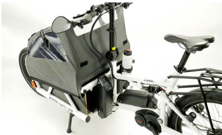
LEFT The Riese & Müller Load touring HS on test had a reserve battery to extend its range. The comfortable handlebar can have its position adjusted without tools. Other practical details include the bottle cage mounts and the frame lock, while the rear suspension adds comfort. A mounting for an additional folding lock is available as an option.
