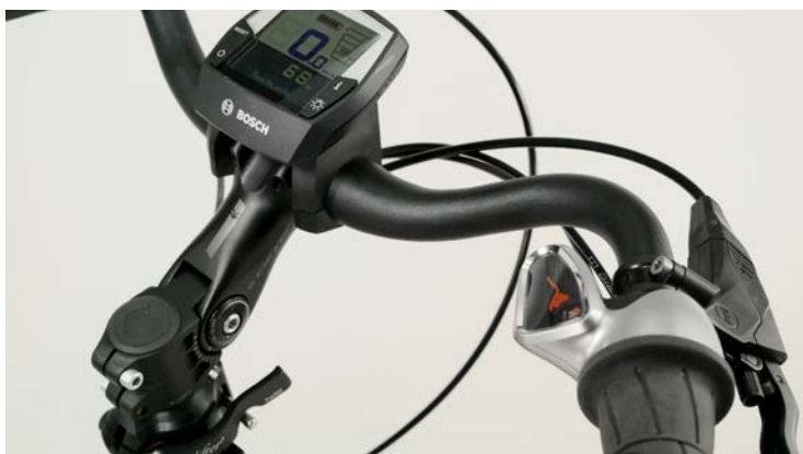
LEFT The stem is designed so that you can adjust the height of the handlebars at will without tools, by opening the quick release. And if you also pull out a safety locking pin, you can then also twist the handlebars around. This is highly practical for parking in narrow cycle lockers or when transporting the bike – be that by train, in a mobile home or on the carrier rack of an intercity bus.
