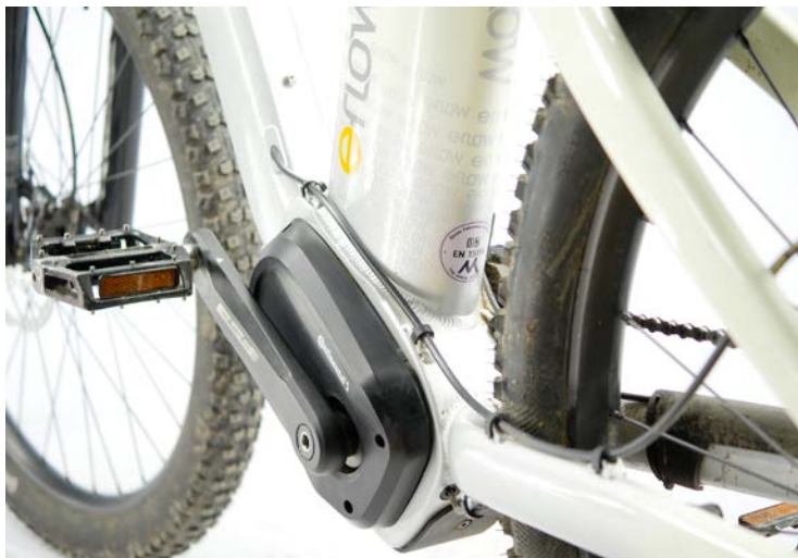
LEFT The Continental mid motor, which is mechanically locked into the frame, runs quiet and smooth. As on many eflow models, the battery pack is hidden in the massive oval seatube. It can be removed along with the saddle and separately height-adjustable seatpost.
