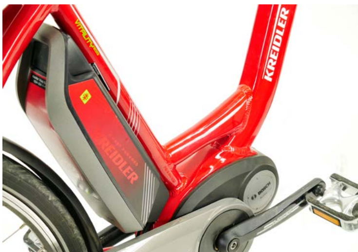
LEFT Practical: the battery pack layout which allows the bike to combine a low centre of gravity with a very low step-through. So it's easy to get on and off this Kreidler Vitality pedelec .
