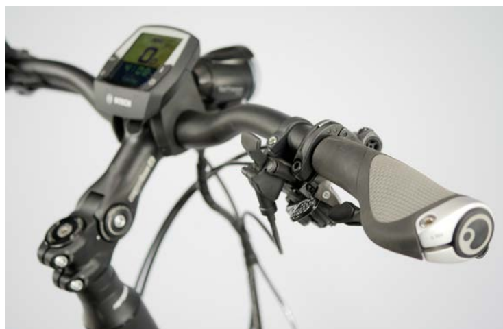
LEFT Comfortable and ergonomic, thanks to the adjustable stem, and grips with large-area palm support. The cockpit looks clean too, with the front light hidden behind the Bosch display in the middle of the handlebars... but this does mean that the space where a handlebar bag or basket would mount is already taken.
