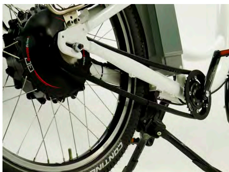
LEFT A powerful motor and the two speeds from the bottom bracket gearbox are perfectly adequate and, together with the chain protected by its plastic sleeve, promise years of low-maintenance service. Operating the two speed gearshift with your heels takes a little getting used to, but after some practice it feels perfectly natural.
