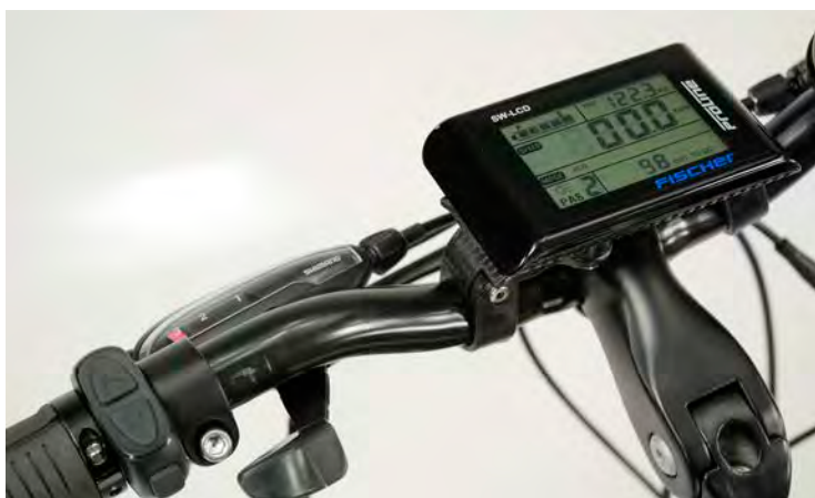
LEFT The cockpit of the Fischer Proline Trekking ETD 1606 , with a multi-functional display mounted fixed to the bike. The USB charge function on the display is self-explanatory and is a must-have for digital nomads. The functions, including the lights, can be easily operated with the thumbs, without taking a hand from the bars. You get masses of functions here for very reasonable money.
