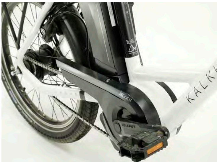
LEFT The Impulse drive is compact, and mounted unobtrusively at the bottom bracket. The battery pack is easily accessible behind the seat-tube, and ensures that the centre of gravity is well placed at the middle of the bike. Test riders praised the frame as stable and nimble.
