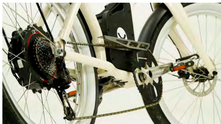
LEFT Distinctive: the bullish white wall tyres and the cream-coloured frame from voluminous aluminium tubes. It all looks rather more solid than is typical for bicycles - and indeed, nothing at all rattles. Double batteries and 500 W hub motor = plenty of power and range. Pure Swiss understatement.
