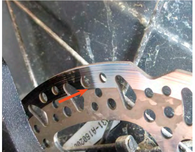
A selection of disasters, mishaps and failures under test: Note that on the picture of the Tektro disk brake on the trioBike cargo bike only part of the braking disk is being used. The reason was that the brake calliper adaptor was mounted the wrong way round (left picture).
