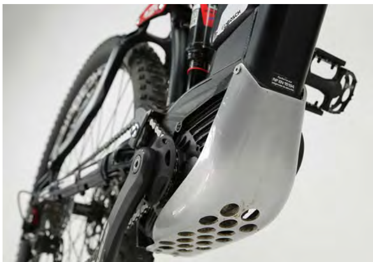
LEFT The mid motor is elegantly and robustly integrated on this Bulls off-road pedelec, and it is far nicer than the original Bosch plastic housing, which in contrast looks cheap. The massive aluminium impact guard gives credible protection to the drive against grounding. It is just a little tedious getting mud out of the holes after riding through it.
