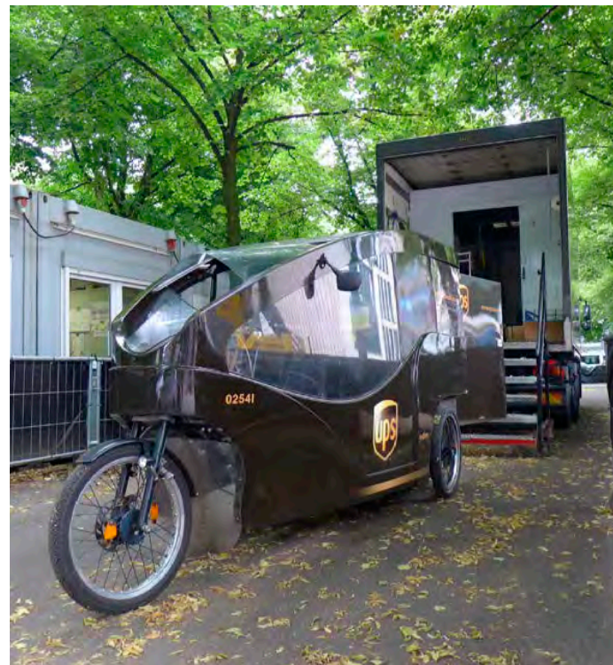
In the city centre of Hamburg, UPS are implementing the combination of container storage areas as micro-depots and deliveries by cargo pedelecs, cargo bikes and handcarts. Pictures is the Cargo Cruiser from Olaf Lange Dreiradbau with a cargo volume of 2.2 m 3 . Photo: Arne Behrensen, cargobike.jetzt
