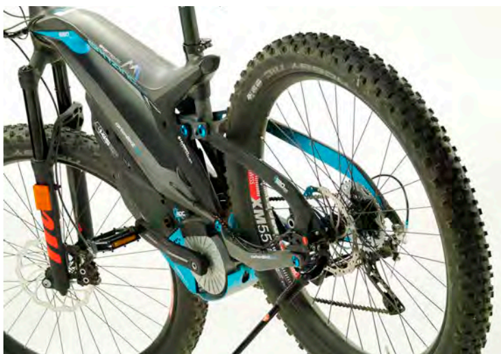
LEFT Because of the very voluminous carbon fibre frame, the knobby tyres on the M1 Spitzing PLUS don't actually look as massive as they really are. Everything about the M1 Spitzing is that bit more powerful, including the mid motor. This, like the bike, is made in the Munich area.
