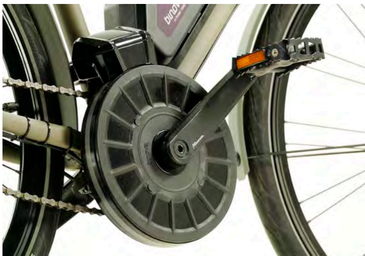
LEFT The flat form factor pedelec motor from Binova , which can be retro-fitted to almost any standard cycle frame. This direct drive motor, which is manufactured in Glashütte in Saxony, provides silent and judder-free assistance.
