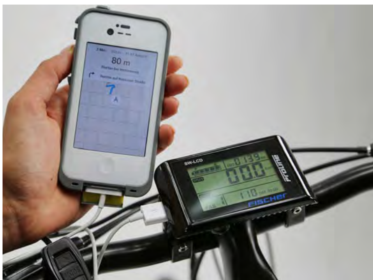
LEFT A very practical detail: the display has a USB port which can be used without adaptors for any standard USB charging cable.
