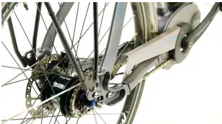
LEFT Simple but functional mass produced technology: Tektro VELA hydraulic disk brakes and the Bosch Active Line mid motor, combined with Shimano Alfine 8 speed hub gear, which sometimes reacts with some delay to gear shifts when climbing, thanks to the built in clutch which prevents shifting under load.
