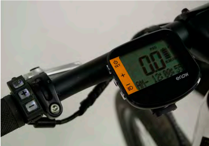
LEFT The removable control unit for the eflow ER2 limits itself to the usual functions of a cycle computer, for example total km, ride km, average km/h, max km/h, and battery capacity and power assist level are also shown. This display is operated with your thumb via a backlit button unit, so you do not have to remove a hand from the handlebars.
