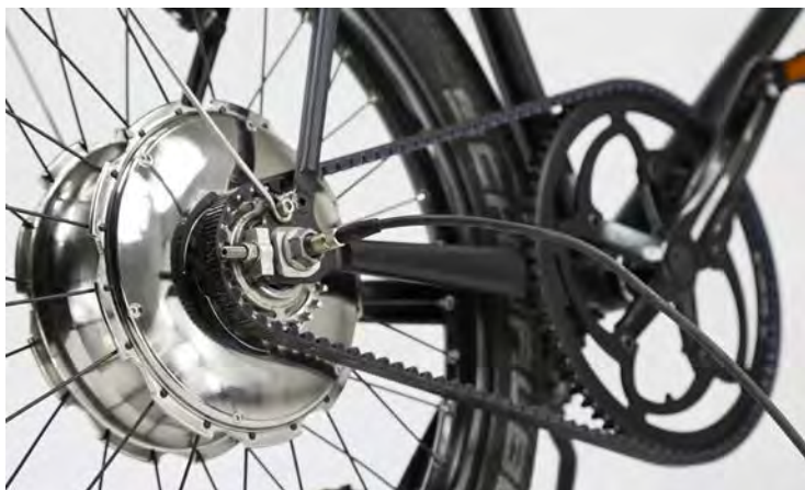
LEFT The Zehus motor fitted to the Klaxon is distinctly out of the ordinary for this ExtraEnergy test. Within its compact shell it incorporates all of the elements of a pedelec drive system: geared motor/generator, batteries, controls and sensors. It also has a charging port, hidden inside a special dome nut into which, when unscrewed, you can plug the charger connector.
