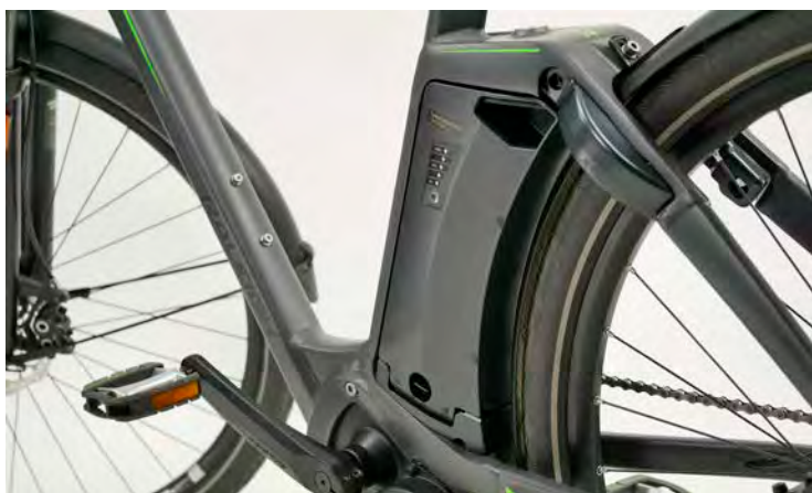
LEFT The Raleigh Ashford is a masterpiece of integration. The battery is placed perfectly between rear wheel and seatpost while frame lock and motor, along with all cables, are integrated into the frame, protected from vandalism. The Rosenberger charging socket, designed for long service life and easy operation, is protected from the external environment by a magnetically-attached cap.
