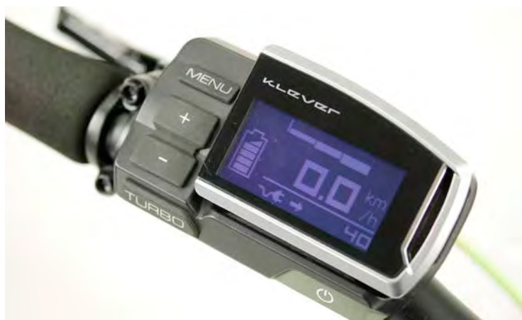
LEFT A fine functional design, the control unit consists of two parts: A) the base unit with the buttons and B) the display unit. This can be quickly attached or removed like a key and stashed away in a trouser pocket. It doesn't jam like some other displays, which firstly are harder to remove and secondly are so large that you're not sure where best to put them.
