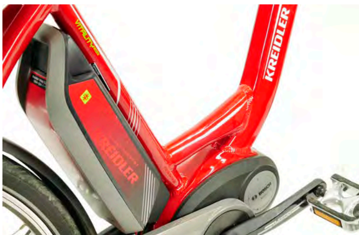
LEFT Practical: the battery pack layout which allows the bike to combine a low centre of gravity with a very low step-through. So it's easy to get on and off this Kreidler Vitality pedelec.
