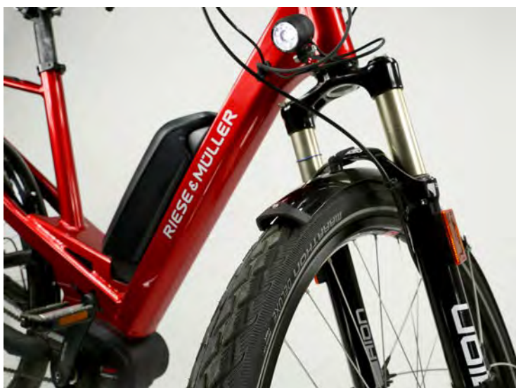
LEFT Full fat: the Schwalbe Marathon Deluxe tyres are a hybrid of the well-proven Marathon model and the comfortable shock-absorbing Big Apple tyres. The Suntour Aion suspension fork has plenty of travel too, and it is equipped with a through-axle system and the orange side reflectors which are mandatory in Germany for pedelecs 45.
