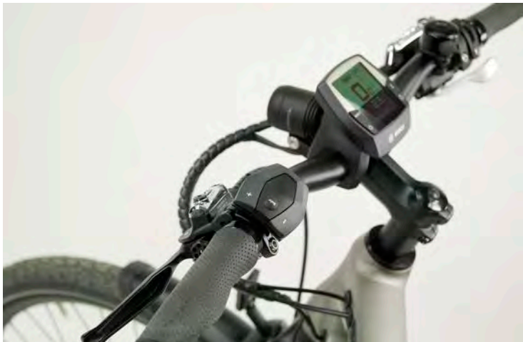
LEFT The cockpit of the Flyer TX 7.70 leaves little to be desired. It comes across as comfortable and tidy: soft, ergonomically-shaped rubber grips, Shimano XT hydraulic brakes and gears, Supernova LED lights, Bosch controls and display components. The overall impression is characteristic of Flyer : top quality materials and components combined with understated colours – traditional values, one might say.
