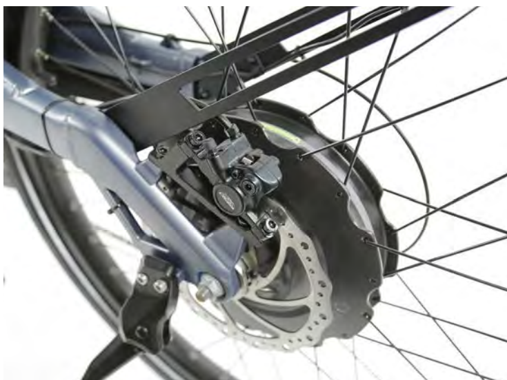
LEFT The Alber motor delivers quiet propulsion. The dropouts and rear stays are, like everything on the Ørsted's frame, custom made.
