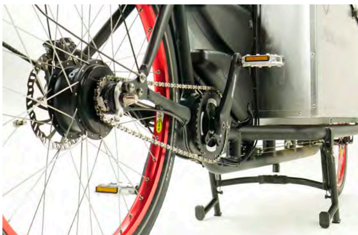
LEFT Masses of technology in not much space: two batteries almost completely fill the frame of the “Pedalpower eHarry”. The “Brose” motor assists your pedalling quietly but powerfully – and the motor power, together with your muscle power, is transferred to the rear wheel by the NuVinci step-less hub gear.
