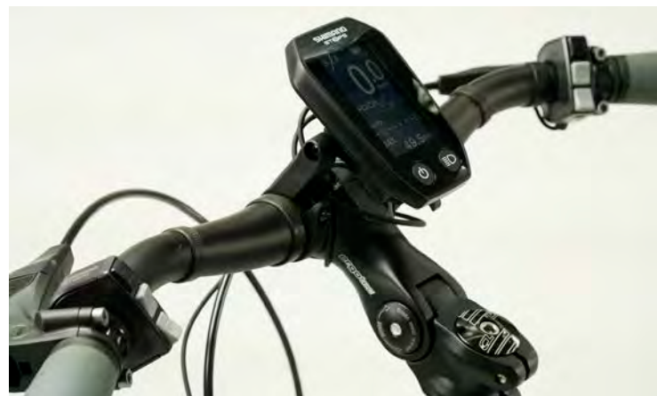
LEFT This pedelec from TRENGA DE appears to have symmetrical user controls on both left and right sides of the handlebars. But test riders quickly discovered that this is a false impression. The two sides control the automatic transmission, which can optionally be shifted manually, and the power assist level.
