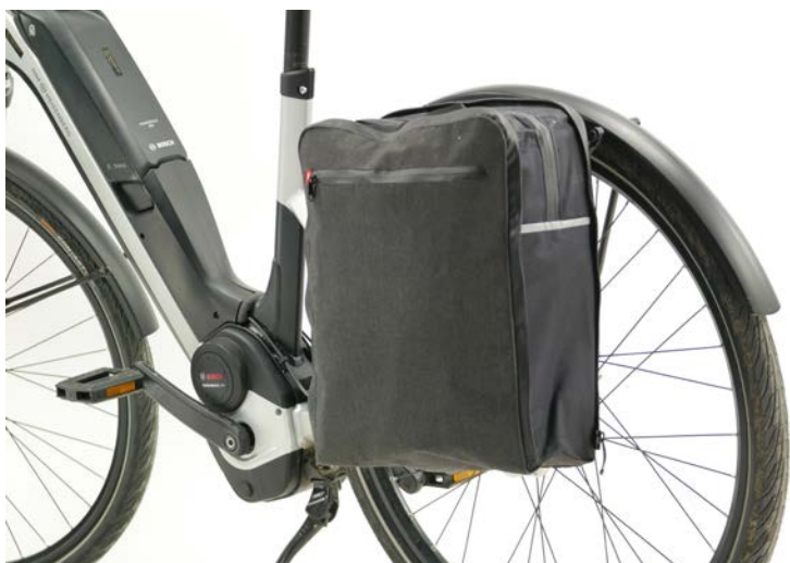
LEFT There's plenty that you can hang on the 'invisible' carrier rack – like the panniers shown here – via the attachment system on the oversized mudguard, which in this case is made from metal, and withstands the loading without any problem. For some things, such as a child seat, you may have to fit a 'classic' carrier rack, or simply use a child trailer instead.
