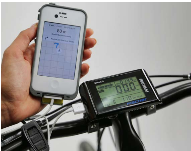
LEFT A very practical detail: the display has a USB port which can be used without adaptors for any standard USB charging cable.
