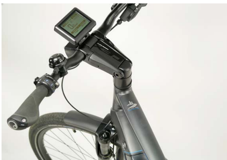
LEFT No rattling or wobbling here. With this model Kalkhoff has managed to make almost all of the hydraulic hoses, wires and Bowden cables, which would otherwise clutter the handlebar area, simply disappear. The stem is massive and similarly massive is the mudguard, made from an extruded aluminium profile – the same technology that is used to manufacture rims.
