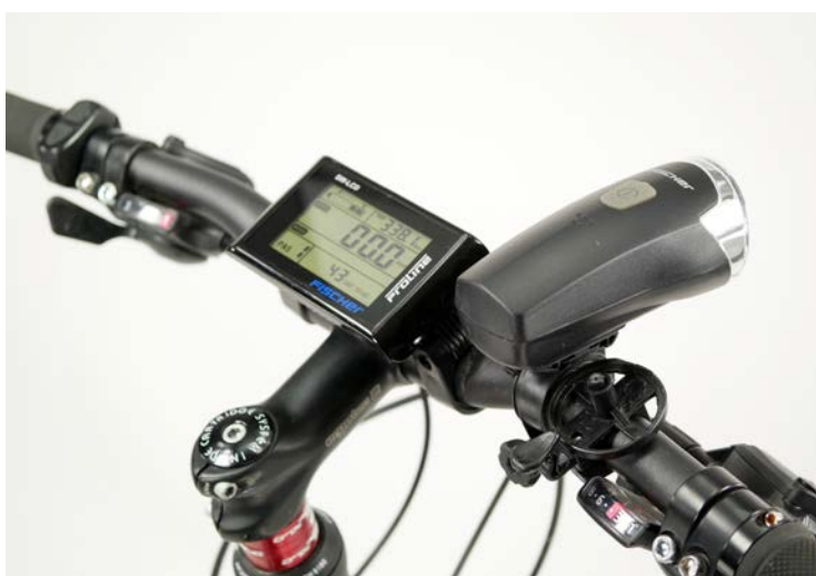
LEFT To retain its clean appearance, for the Proline EM 1614 offroad pedelec Fischer supplies 50 Lux LED detachable lights and spoke reflectors, which can be easily fitted or removed as required. The very basic bell removed itself. The almost identical but cheaper sister model, the Proline MTB EM 1608 , is supplied without lighting set, with a smaller battery and with different warranty terms for a RRP of 1399 Euro. Details of how to order are at: www.fischer-die-fahrradmarke.de
