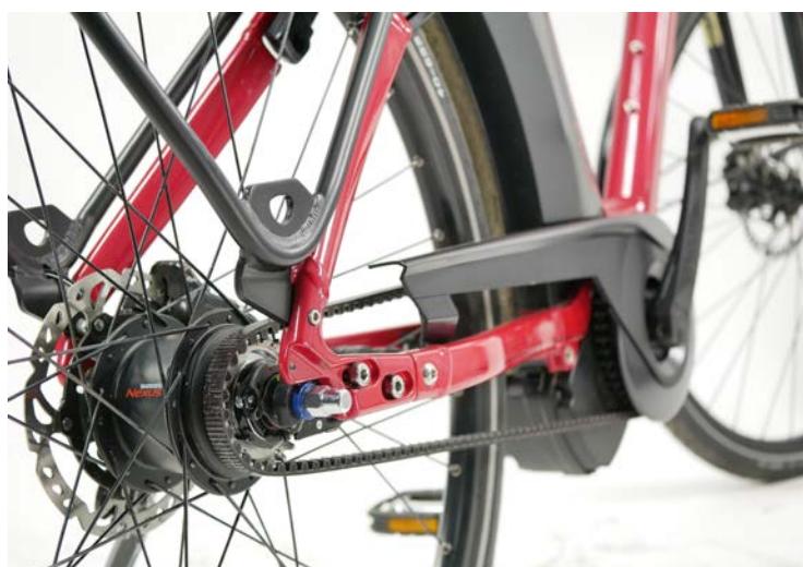
LEFT The creativity of the Kalkhoff developers is demonstrated, for example, by the manner in which the carrier rack is joined to the frame via the dropouts. The plates which support the carrier rack legs on each side locate into grooves in the frame, so that the load is transmitted directly to the frame itself. This means that the forces are not, as is usually the case, pressing on the attachment bolts, which can lead to swift fatigue failure.
