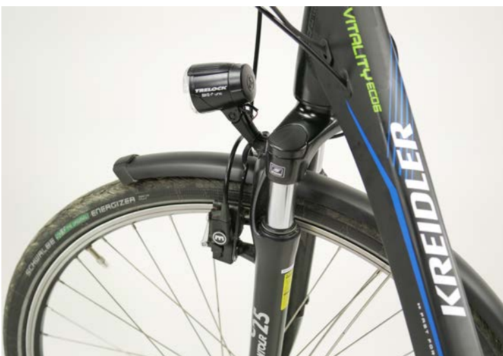
LEFT The Kreidler Vitality ECO6 is a good example of how component manufacturers are taking pedelecs ever more seriously, and how they are manufacturing parts specifically for these vehicles. Here there's a pedelec 25 specific fork from the world market leader in mid-priced suspension forks, plus tyres from Schwalbe specially developed for pedelecs.
