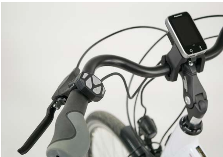
LEFT Height-adjustable stem, swept-back handlebars and ergonomic grips were all appreciated by the testers. The Magura hydraulic rim brakes provided good stopping, with silky-smooth modulation. The central display for the power assist system has a USB port to supply power to other electrical devices, for example a mobile phone or a GPS navigation system.
