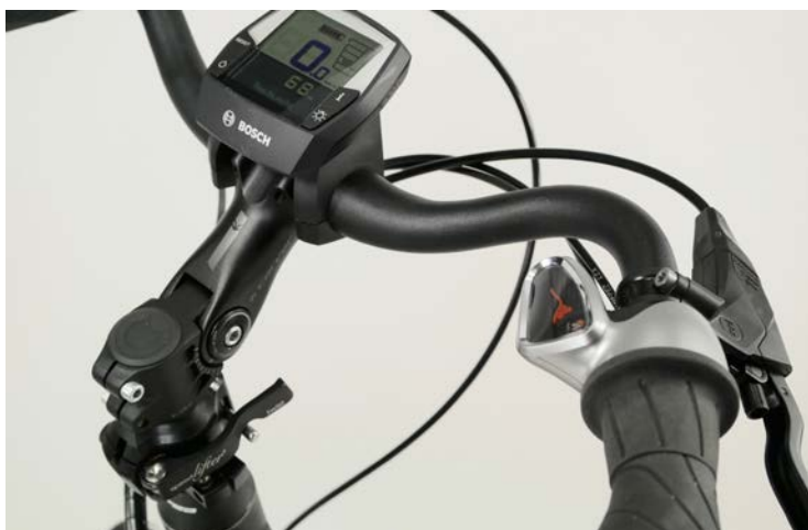
LEFT The stem is designed so that you can adjust the height of the handlebars at will without tools, by opening the quick release. And if you also pull out a safety locking pin, you can then also twist the handlebars around. This is highly practical for parking in narrow cycle lockers or when transporting the bike – be that by train, in a mobile home or on the carrier rack of an intercity bus.
