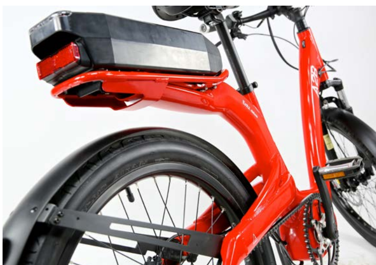
LEFT The frame of the Entz Deluxe is an imposing and distinctive design, finished here in an appropriately high-contrast red. It's hard to believe that such flowing lines can be formed from tubing, and indeed to build this frame they have used much hydroforming of tubing, milling of tubes and stock materials, and hand-finishing of weld seams.
