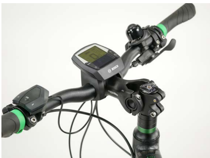
LEFT That this bike is intended for heavier loadings is evident in the adjustable stem – it is clearly rather more generously dimensioned than is usual. There are ergonomic grips, and the rider will quickly grasp the functions of the rest of the controls, from Bosch and Shimano, and rapidly learn to operate them intuitively.
