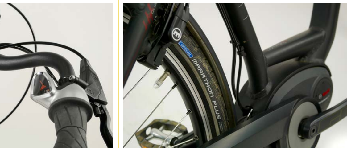
RIGHT Schwalbe Marathon Plus tyres with, according to the Schwalbe factory, the toughest puncture-resistant protective layer on the market. Fitted on the Carver Cityzen 1050 is the E-Bike Ready 50 version, designed for use in pedelecs 45. This is an example which shows how Carver haven't just concentrated on the bare technical necessities in specifying the Cityzen 1050; instead they've often gone an extra mile.
