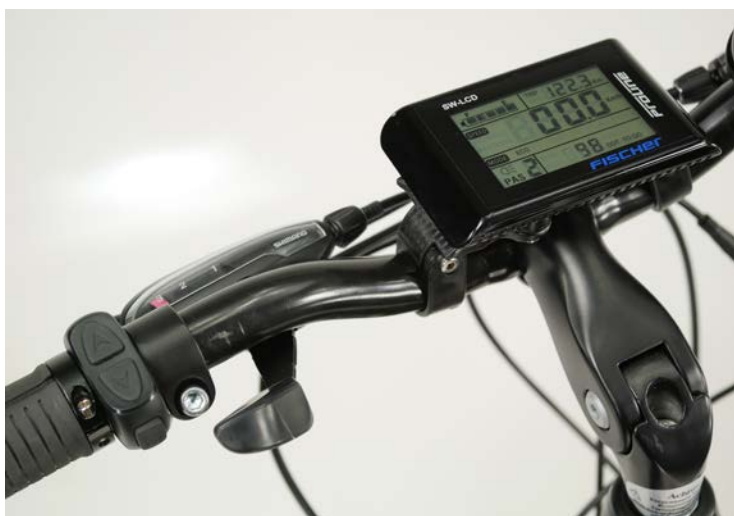
LEFT The cockpit of the Fischer Proline Trekking ETD 1606 , with a multi-functional display mounted fixed to the bike. The USB charge function on the display is self-explanatory and is a must-have for digital nomads. The functions, including the lights, can be easily operated with the thumbs, without taking a hand from the bars. You get masses of functions here for very reasonable money.
