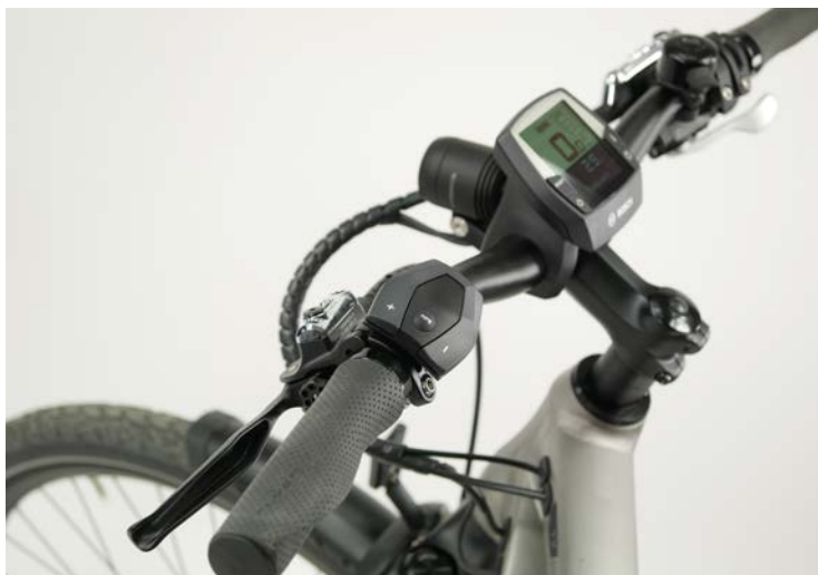
LEFT The cockpit of the Flyer TX 7.70 leaves little to be desired. It comes across as comfortable and tidy: soft, ergonomically-shaped rubber grips, Shimano XT hydraulic brakes and gears, Supernova LED lights, Bosch controls and display components. The overall impression is characteristic of Flyer: top quality materials and components combined with understated colours – traditional values, one might say.
