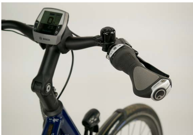
LEFT Comfortable, robust and tidy: the cockpit of the Hercules Futura F8 . It's just what you might imagine for a bike for everyday use: no bells and whistles, yet everything essential to hand. The ergonomic grips provide a secure and comfortable grip on the bars. In everyday use one might wish for a display which you do not always need to take with you, so as not to worry that it will be stolen.
