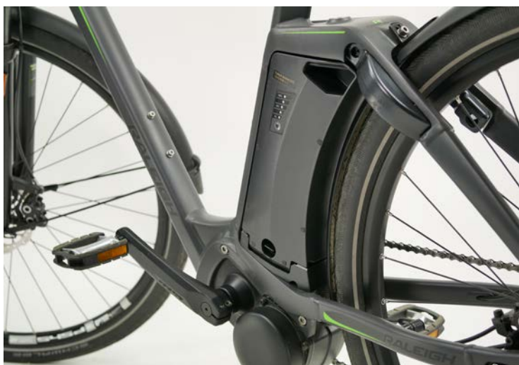
LEFT The Raleigh Ashford is a masterpiece of integration. The battery is placed perfectly between rear wheel and seatpost while frame lock and motor, along with all cables, are integrated into the frame, protected from vandalism. The Rosenberger charging socket, designed for long service life and easy operation, is protected from the external environment by a magnetically-attached cap.
