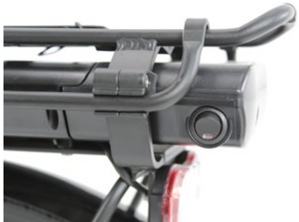
LEFT From the outside, the battery pack, made by Ansmann, looks like a replica of a Chinese battery pack. The rocker switch to turn on the pack can at times be confusing in operation; it’s sometimes still at „On“ when the battery is actually off – this occurs when the battery has switched itself off through lack of use.
