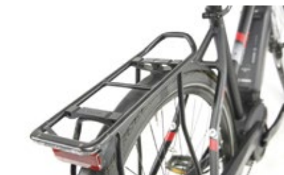
LEFT The Racktime carrier rack on the Pegasus Premio E10, with its attachment system, might have been made for mounting a childseat or for securing bags of shopping. It's good for higher loads on the carrier rack that the 2.4 kg battery is positioned well towards the front of the bike. The rear-mounted stand gives improved weight distribution and good parking stability.
