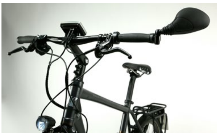
LEFT The Endeavour S11 is, as a Pedelec 45, equipped as befits a powered vehicle with items including a rear view mirror, side reflectors, brake levers with rounded rather than sharp ends, and number plates. It is a practical touch that both display and saddle can only be removed using tools. Nonetheless a switch-on lockout would also be useful, for example authenticating the user via NFC or Bluetooth
