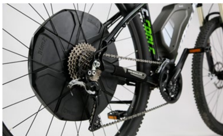
LEFT A completely new generation of BionX motor, with a plastic housing and now no risk of overheating on long, steep ascents. It gains its torque from the lever arm of its large diameter and so as with the previous generation it operates without any gears. The motor delivers its power very directly, but it is not at all jerky: just what you would expect from a BionX system.
