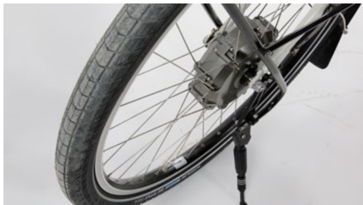
LEFT The front wheel motor has a housing from Chinese manufacturer Crystalite, but according to Utopia the internals, windings and electronics are all made in the Netherlands.
