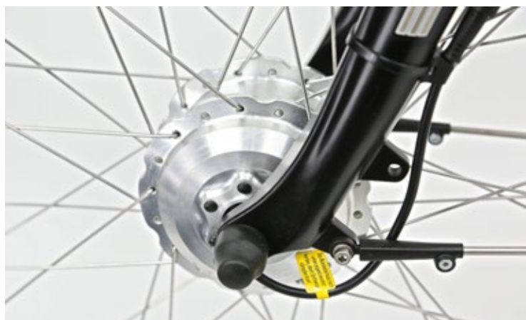
LEFT The Ansmann front hub motor excelled in the tests with its unique power density: it is small, but very powerful and also whisper quiet. The yellow warning label on the cable is also interesting: it notes that water could seep into the motor if the cable does not have a downwards loop from which water running along the cable can drop off.
