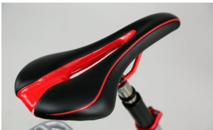
LEFT The saddle on the Kettler Traveller E-Light looks 'uncomfortably sporty' but in fact, it was rated by the test riders as rather comfortable, helped no doubt by the good suspension seatpost. As on almost all of the other components too, red colour highlights decorate the saddle and seatpost clamp.
