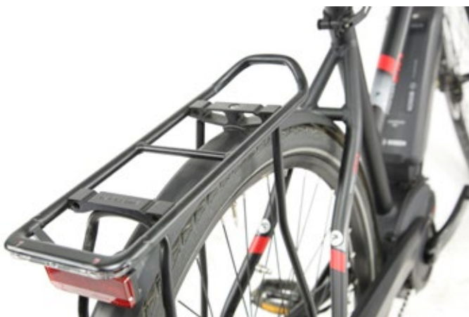
LEFT The Racktime carrier rack on the Pegasus Premio E10, with its attachment system, might have been made for mounting a childseat or for securing bags of shopping. It's good for higher loads on the carrier rack that the 2.4 kg battery is positioned well towards the front of the bike. The rear-mounted stand gives improved weight distribution and good parking stability.
