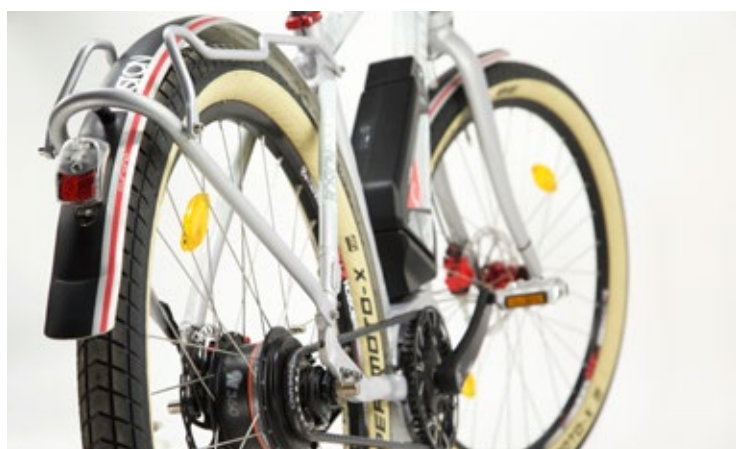
LEFT The Kettler Boston is lovingly decorated down to the finest detail with graphics and logos, rather like a mobile billboard. Nonetheless, the technology is state of the art. No expense has been spared: Gates belt drive, stepless hub gearing and balloon tyres. The carrier rack is also interesting: it lets you carry panniers, while visually it's as if it weren't there at all.
