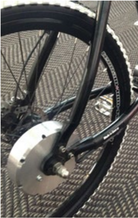
An example of a fully-digital chainless drive. Pictured here is a functional prototype, which actually operates very well, from German manufacturer Mifa .
