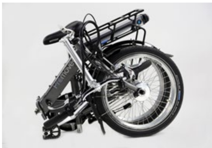
LEFT Folded up, at 81 x 49 x 75 cm (L x W x H) the Pro-Movec folding pedelec is a very easily handled package, and a useful aid to 'multimodal transport': taking it with you by bus or train, or for a quick ride from a cheap parking spot to your destination.
