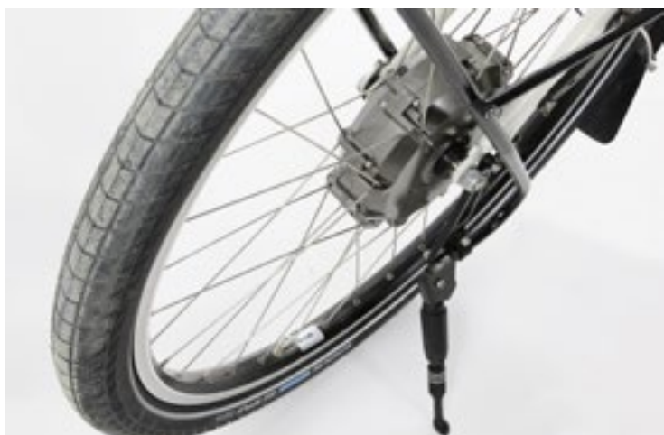
LEFT The front wheel motor housing is from Chinese manufacturer Crystalite , but according to Utopia the internals, windings and electronics are all made in the Netherlands.
