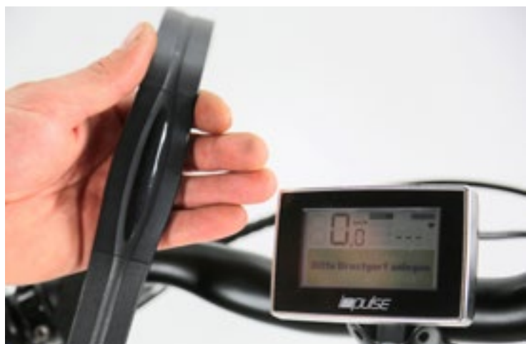
LEFT The Impulse drive from Daum electronic can vary the assist level according to the rider's heartrate. Currently a chest strap is used to measure the pulse rate, but in future this function will become easier to fit into the daily routine, using Bluetooth connectivity for example.
