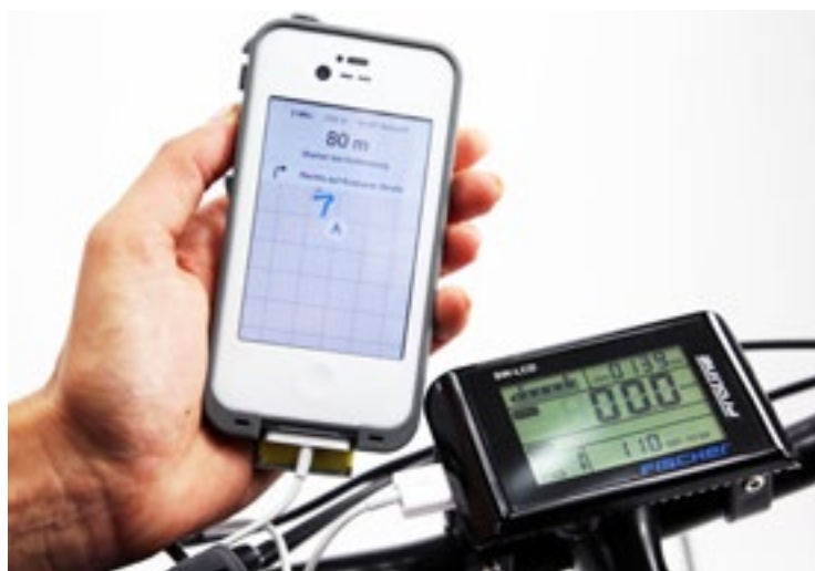
LEFT A very practical detail: the handlebar display incorporates a USB port which can be used without adaptors for any standard USB charging cable.
