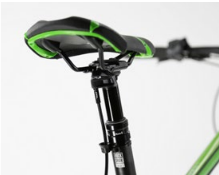
LEFT Practical off-road and for touring: the saddle height adjustment controlled from the handlebars.
