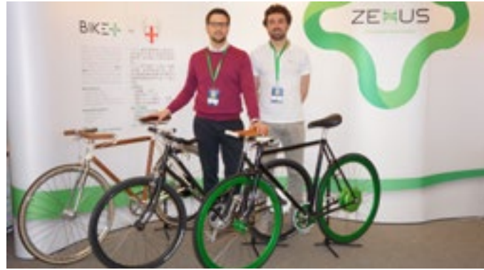
Ivo Boniolo and Giovanni Ali from the Italian company Zehus exhibited their revolutionary Zehus Pedelec System at the China Cycle Show in April 2014. It breaks completely new ground electronically, and doesn't involve a single cable on the bike's frame – and it also doesn't need a charger, because it extracts energy from the rider's pedal power at moments of optimum biomechanical efficiency and uses this to charge the battery within the motor housing. Then this energy can be used at times of low human pedalling efficiency by being converted back by the motor into mechanical power assistance.
