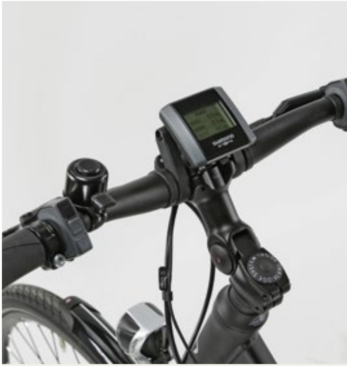
Handlebars with Shimano's pedelec system — Shimano's trump card for its entry into the pedelec mid motor market is its combination of mid motor and electrically-operated gear shifting. The system, of their own manufacture, eases off the power of the mid motor for an instant at the moment when the gear shift occurs.
