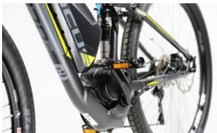
LEFT The drive system, made by daum electronic of Fürth, Germany, shows what it's capable of in the Thron . Being fitted above the downtube means that it's exceptionally well protected against grounding, for example when jumping over logs or boulders.
