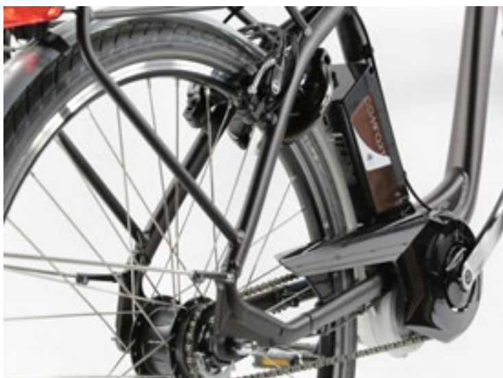
LEFT As with previous models in the Obra series, Kettler has opted for proven technology including the Panasonic mid motor and Magura rim brakes.
