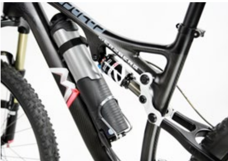
LEFT The M1 is a master of disguise: from a distance it looks just like a full-suspension MTB with an oversized alloy frame and drinks bottle. On closer inspection you notice the elaborate carbon frame, and what looks like a drinks bottle is revealed as a battery.
