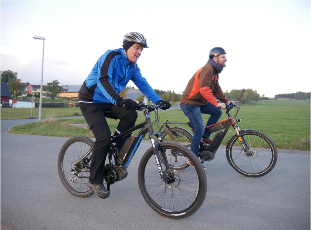
*On the final section the test riders switch off the motor, so as to rate the ride performance of the test bikes without motor assistance. Picture: Angela Budde (editor, [ExtraEnergy.org](http://ExtraEnergy.org))*
