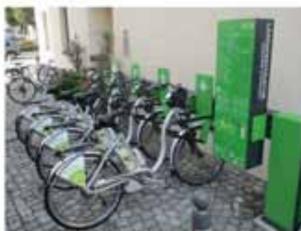
The first shared public charging and leasing infrastructure, installed by EnergyBus member ibi in 2011. It allows the charging of each bike station with the EnergyBus connector.
